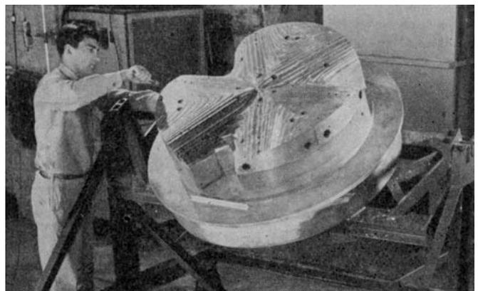
Figure 3: One of the magnet poles for the second electron model sector-focused cyclotron.
