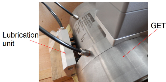
Figure 5: GET with modified pressure-resistant lubrication unit. The lubrication unit must be operated manually
