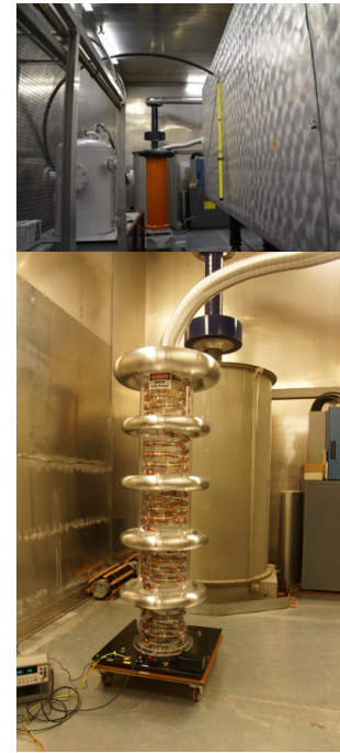
Figure 5: The Faraday room of the electron cooler. Top: The -320 kV power supply is shown on the left and the HV platform on the right. The HVDC2.1 200 kV (2 G \Omega ) DC HV divider (property of the PTB) is installed (in orange). Bottom: The Ohmlabs HVS 250 kV (250 M \Omega ) DC HV divider (property of the TU Darmstadt) specified for 10^{-4} precision is installed. The isolating transformer (in grey) powering the HV platform is seen in the back.
