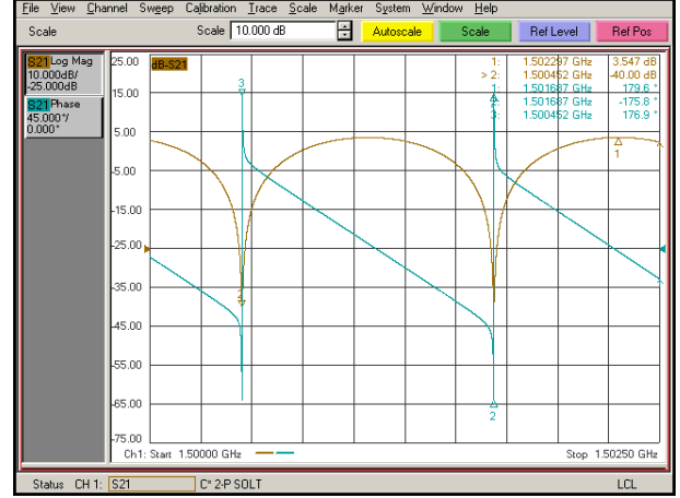
Figure 6: Measured response of the notch filter close to 2 notches at midband (1.5 GHz). The notch distance is 1.235 MHz. Because of the finite notch depth, the phase jump at each notch was less ( 177^\circ ) than the 180^\circ expected in the ideal case. The variable attenuator was set at 0.99 dB. (Due to temperature dependence of the setup later measurements vary in attenuation.)
