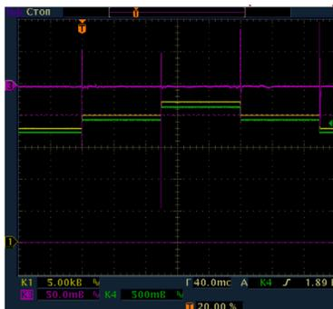
Figure 4: Signal from test-bench, the pulse amplitude  $\pm 2$  kV, the voltage of the main power supply is 20 kV.
