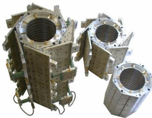
Figure 3: PU / KI of the high energy SC system for HESR. Right: One stack of 16 slot rings. Center: eight combiner boards are attached to the electrode lines. Right: Two stacks, boards are combined pairwise.
