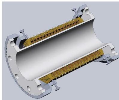
Figure 2: Schematics of pickup (kicker) with internal sealing using ceramic vacuum chamber.
