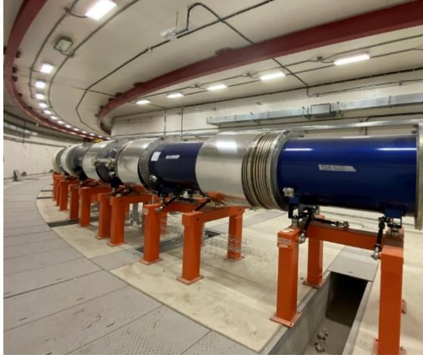
Figure 9: Assembling of Collider arc magnets.
