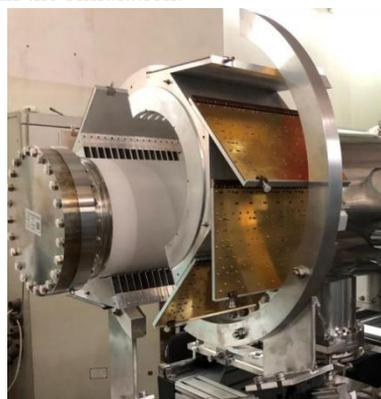
Figure 9: Photograph of the 16 slot-ring cells structure, with 16-way Wilkinson stripline combiner-boards and an 8 mm thickness ceramic vacuum chamber.
