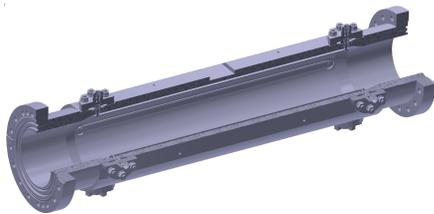
Figure 11: 3D model of the HEL BPM prototype.
