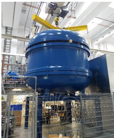
Figure 2: “Big-Blue-Bubble” HV tank with several ports in the bottom flange. Besides the input/output port for the cooler beam, the bottom flange also comprises input/output ports for the gas flow.
