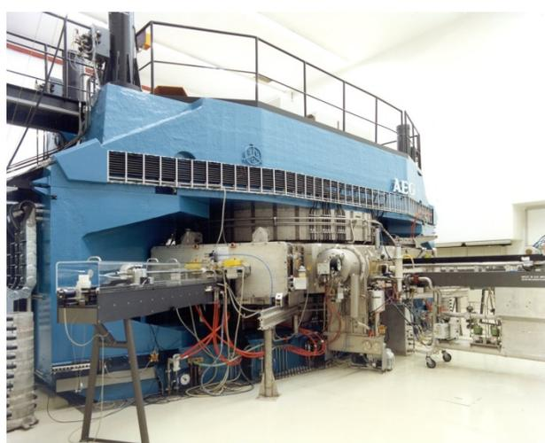
Figure 1: The isochronous cyclotron JULIC.
