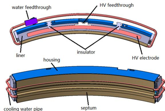
the cooling water pipe is brazed in the groove to achieve the best cooling effect.
