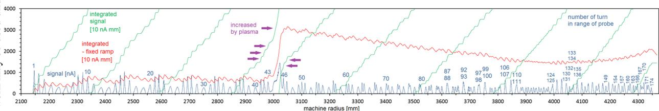
Figure 2: A nicer example of a measurement taken at a beam current of 2200  $\mu\text{A}$ . It is affected by plasma only in a narrow range. A day later, the maximum disturbance was 30 times larger and affected many more turns. With the beam switched off but RF still on, the artefact from the plasma cloud decays within seconds.
