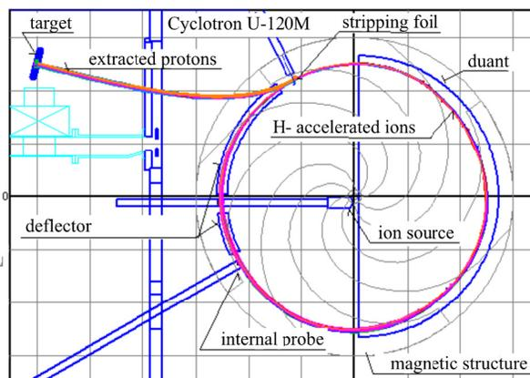
Figure 1: Schematic diagram of U-120M cyclotron with deflection and extraction system.
