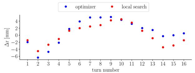
Figure 2: Error of the turn radius at RRI2 between measurement and simulation of the best individual obtained by multi-objective optimization and local search.
