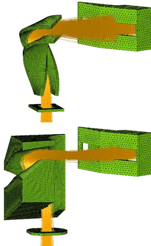
Figure 1: Beam passing through the inflector and striking the vertical slit in an ordinary spiral inflector (top), and in a field gradient inflector with vertical focussing (bottom).
