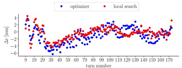
Figure 3: Error of the turn radius at RRL between measurement and simulation of the best individual obtained by multi-objective optimization and local search.
