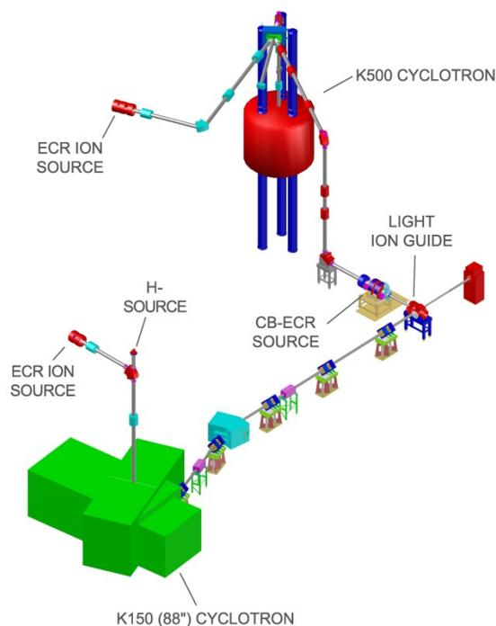
Figure 1: Simplified layout of the Texas A&M light-ion-guide scheme.
