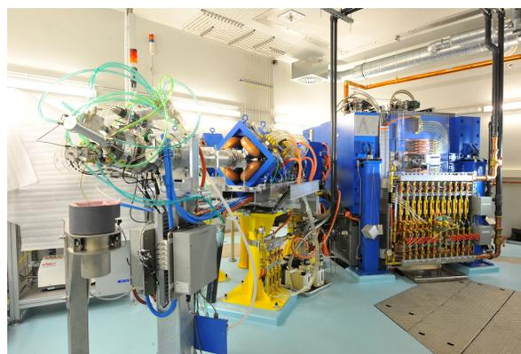
Figure 1: The TR-Flex cyclotron at the HZDR. The beamline 1B with a 4-port target selector is shown in the foreground. The second 4-port target selector is at the opposite side of the Cyclotron.
