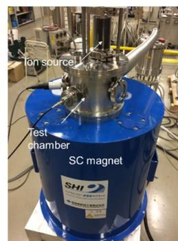
Figure 2: Test bench of ion source.
