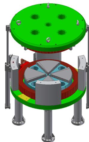
Figure 2: 3D drawings of cyclotron for AMS.
