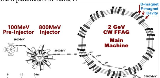
Figure 2: The layout of the circular accelerator complex.
