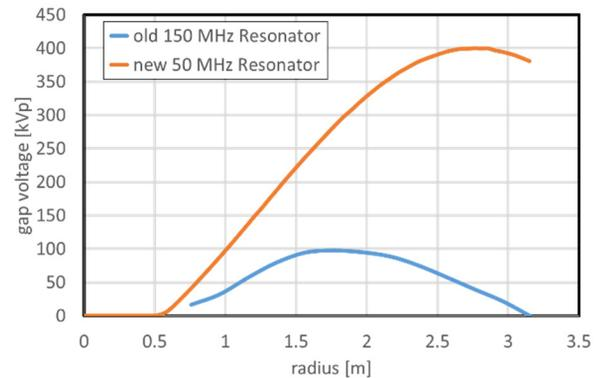
Figure 1: Gap voltage of Resonators 2 & 4.
