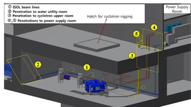
Figure 1: Penetration holes and a hatch in the cyclotron vault and in the upper room. The vault is located in B1. In ④ there are holes for rf transmission line of the final amplifier located in the power supply room, which is not needed for the IBA cyclotron.
