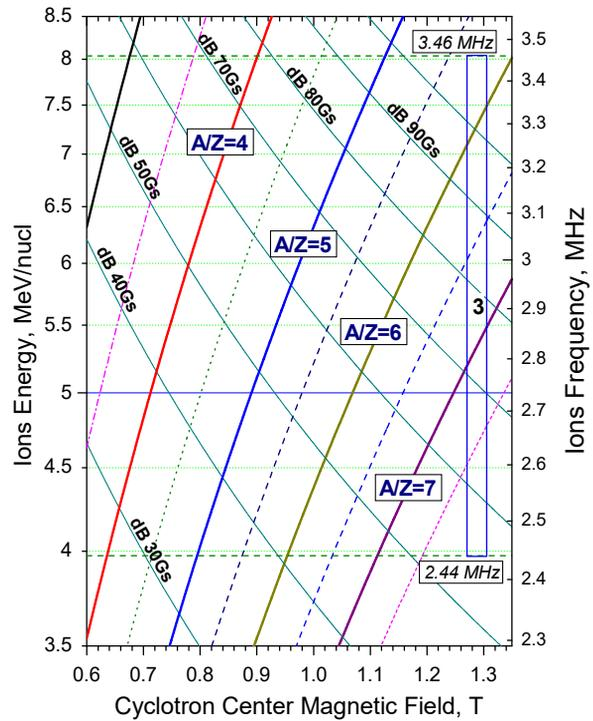
Figure 1: DC-280 Working diagram.
