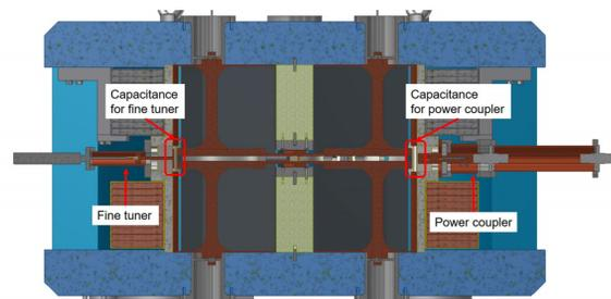
Figure 1: Power coupler and fine tuner for SKKUCY-10.
