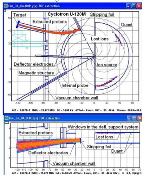
Figure 1: TOF extraction system arrangement.
