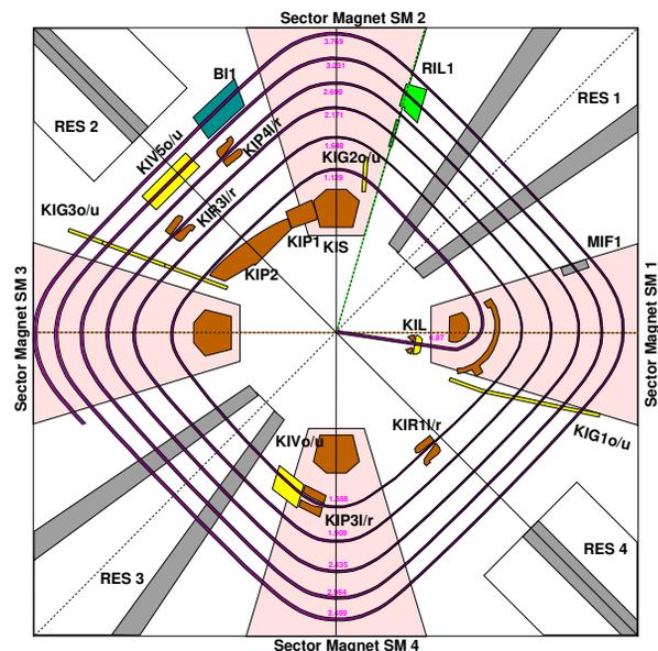
Figure 1: Layout of the central region of Injector 2.
