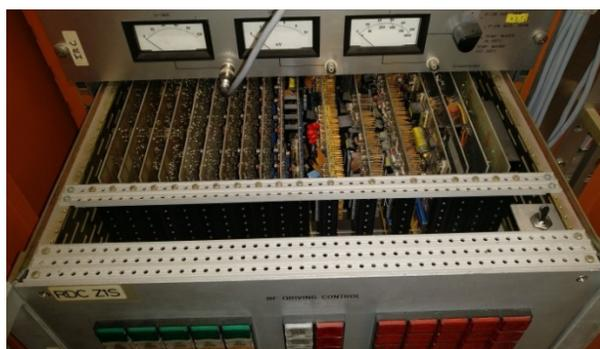
Figure 1: Old low level RF control system.
