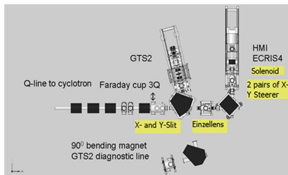
Figure 1: Experimental layout for the oven and MIVOC experiments.
