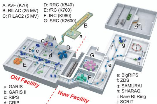
Figure 1: Schematic drawing of the RIKEN RI Beam Factory (RIBF). The accelerators (A–G) and experimental devices (a–j) are presented.
