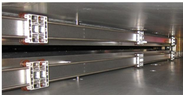
Figure 1: Actual probe fully inserted. The last trolley to the left (not shown) which combines upper and lower arm of the fork stays in the outer chamber. Some of the seven fixtures of the rails are visible.
