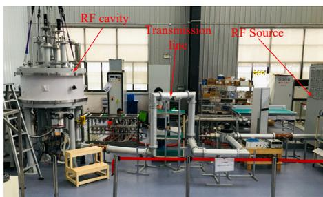
Figure 1: Assembled RF system in commissioning stage.
