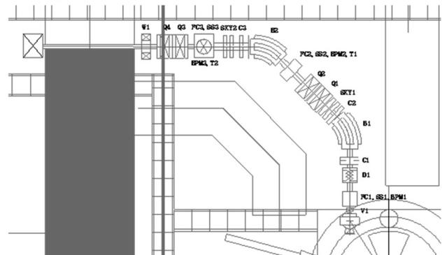
Figure 1: The layout of the 50 MeV beam transfer system.
