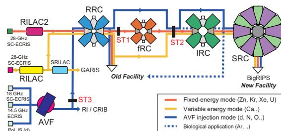
Figure 2: Accelerator chain of the RIBF. The three injectors, RILAC2, RILAC, and the AVF cyclotron, are followed by four booster cyclotrons, the RIKEN Ring Cyclotron (RRC), fixed-frequency Ring Cyclotron (fRC), Intermediate-stage Ring Cyclotron (IRC), and Superconducting Ring Cyclotron (SRC). The charge strippers are indicated by labels in red text (ST1–ST3). The superconducting linac booster, SRILAC, is under construction [3].
