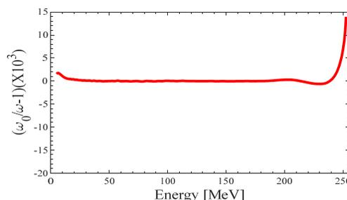
Figure 1: The isochronism parameter  $(\omega_0 / \omega - 1)$  vs. energy.
