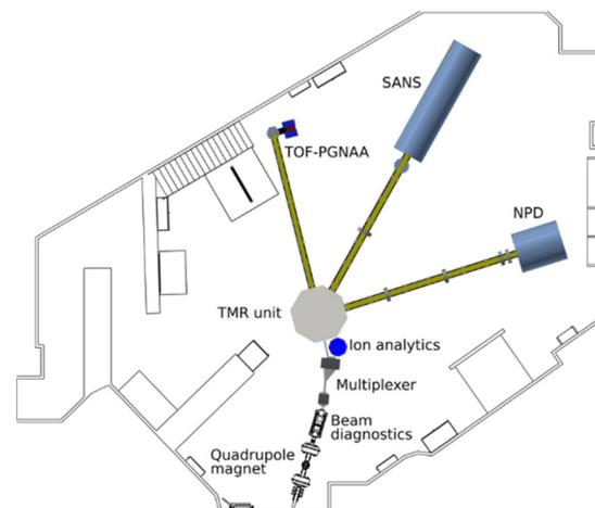
Figure 2: Planned experimental setup in Big Karl area.
