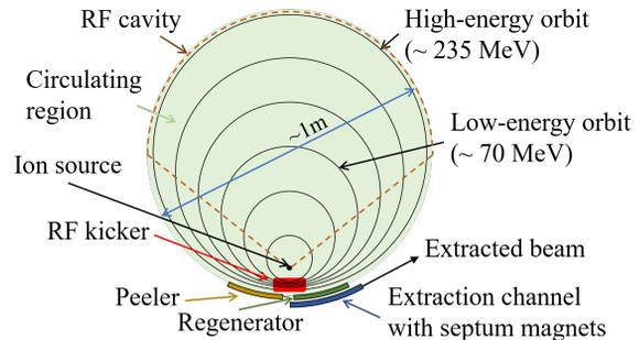
Figure 1: Schematic of compact accelerator.
