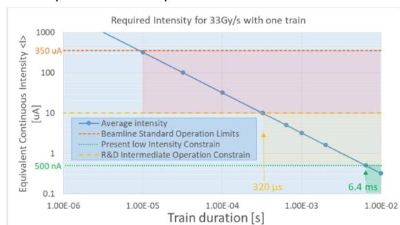
Figure 1: Avg. intensity as a function of the train duration to reach a dosimetry of 33 Gy/s at the Bragg peak plateau.
