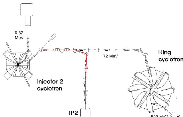
Figure 1: The beam transfer from the Cockroft Walton accelerator via the Injector II cyclotron to the Ring cyclotron. The red line indicates the 72 MeV beam gleaned from Injector II to IP2. Figure adapted from [2].
