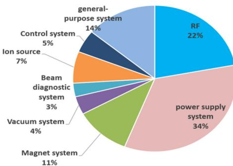
Figure 3: Average failure ratio of the accelerator subsystem during the recent five years.
