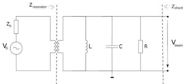
Figure 1: RLC equivalent circuit of a RF system. Adapted from F. Caspers [1].
