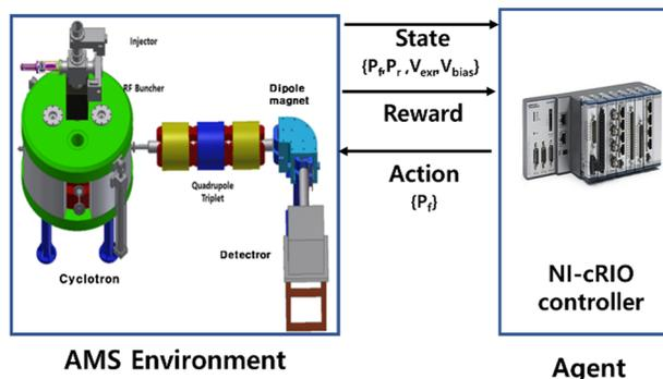
Figure 1: Reinforcement Learning based AMS control block diagram.
