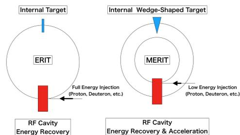
Figure 1: Schematic diagram of ERIT and MERIT scheme.
