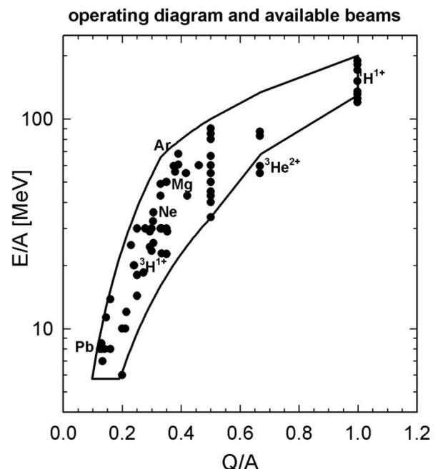
Figure 1: Operating diagram of the AGOR cyclotron.
