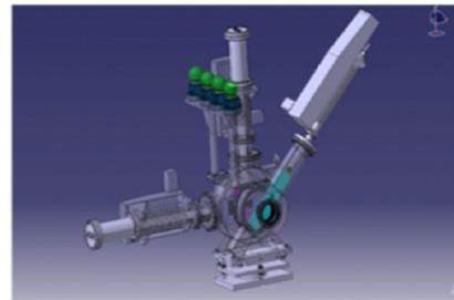
Figure 3: The emittance meter of LINAC4.
