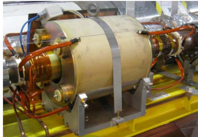
Figure 2: The DCCT with the connexions for the beam intensity measurement.
