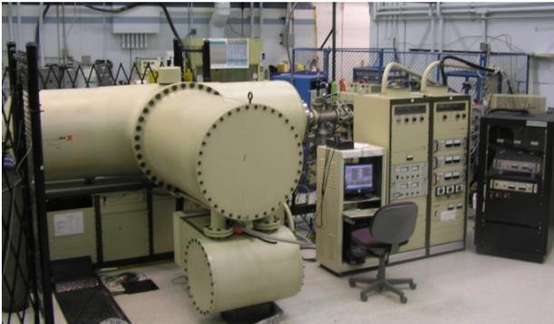
Figure 1: 1.7 MV Tandetron accelerator.
