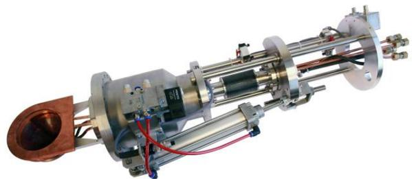
Figure 2: Photograph of the Faraday Cup of the L.E.B.T.
