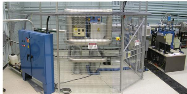
Figure 2: 2 NEC's 400 kV ion implanter.
