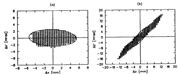
Figure 1: Acceptances of the RTM, and approximated ellipses from linac emittance measurements.
