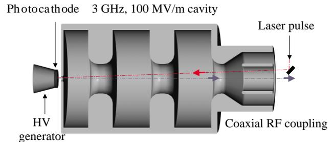
Figure 1: Schematic of the DC/RF gun
