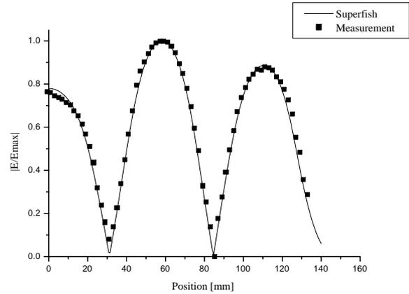
Figure 5: Measurement and Superfish simulation of the on axis field profile in the cavity
