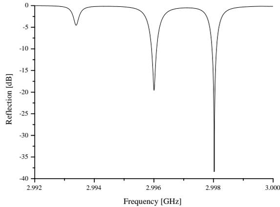
Figure 4: Resonance frequencies of the cavity
