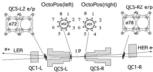
Figure 1: The schematic view of BPMs in the interaction region. Two OctoPos BPMs(left and right side of I.P.) are located between the super conducting quadrupoles, in the longitudinal field of the BELLE detector.
