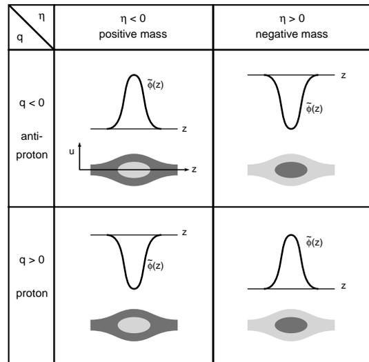
Figure 1: The dimensional electric potential  $\tilde{\phi} \sim \eta q \phi$  as a function of space and the corresponding phase space pattern for four different cases ( $q$  is the particle charge,  $\eta$  is the slip factor). In brighter phase space regions the distribution function is less dense.
