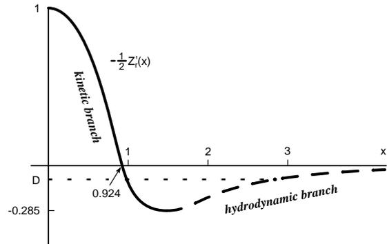
Figure 2: The real part of  $-\frac{1}{2}Z'(x)$ ,  $Z(z)$  being the plasma dispersion function, as a function of  $x = Rez$ .
