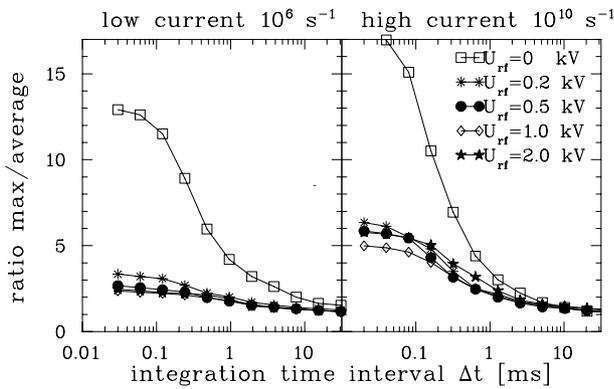
Figure 3: The ratio of maximum-to-average current for a 300 MeV/u Ar<sup>18+</sup> beam using various bunching voltages as a function of the integration time. Results for low current ( $\sim 10^6$  s<sup>-1</sup> using a scintillator) on the left and high current ( $\sim 10^{10}$  s<sup>-1</sup> using the CCC) are displayed.
