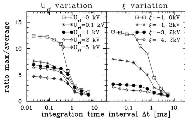
Figure 5: The ratio of maximum-to-average current as calculated for a 300 MeV/u  $C^{6+}$  beam as a function of the integration time. On the right  $\xi = -1$  (corresponding to the normal SIS setting), on the left the proposed improvement for different  $\xi$  are shown.
