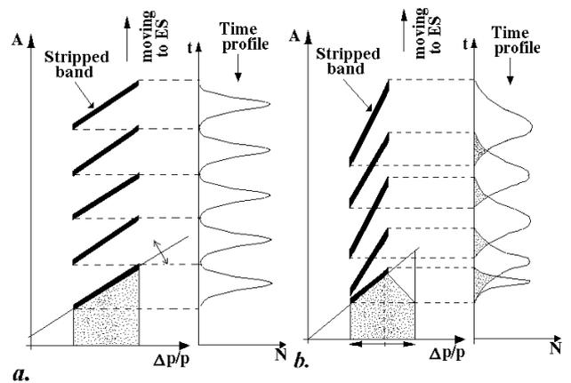
Figure 6: Steinbach-diagram to visualize that the flux of particles is obtained by summing over the 'strip profiles' without bunching (left) and with bunching (right).
