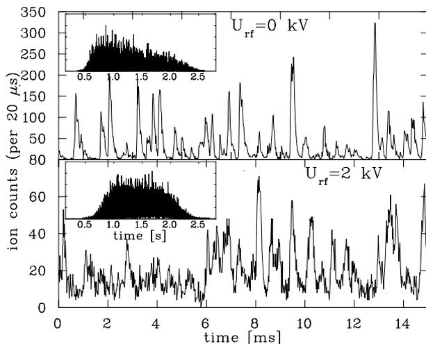
Figure 1: Typical time structure of a spill extracted by tune variation without bunching (top) and improvement by a 2 kV bunching voltage (bottom). The full spill-signal of the 300 MeV/u  $\text{C}^{6+}$  beam is drawn in the insert.
