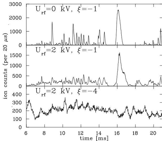
Figure 4: Simulated time structure of a spill extracted by tune variation without bunching and chromaticity  $\xi = -1$ , like at SIS (top), with bunching using 2 kV (middle) and improved structure using bunching and  $\xi = -4$  (bottom).
