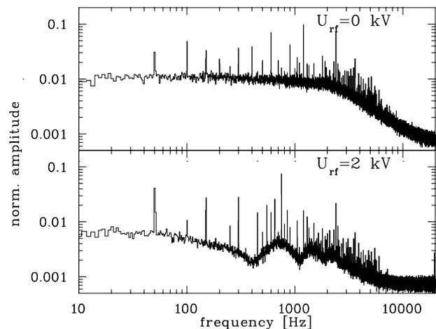
Figure 2: Fourier transformation of the signals displayed in Fig.1 averaged over 10 Spills; without bunching (top) and with bunching (bottom).
