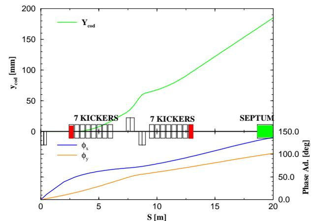
Figure 2: The  $y_{\text{cod}}$  (top) and  $\phi_{x,y}$  (bottom) along the straight section. Two more kickers (red boxes) are needed to extract a 1.3 GeV proton beam.
