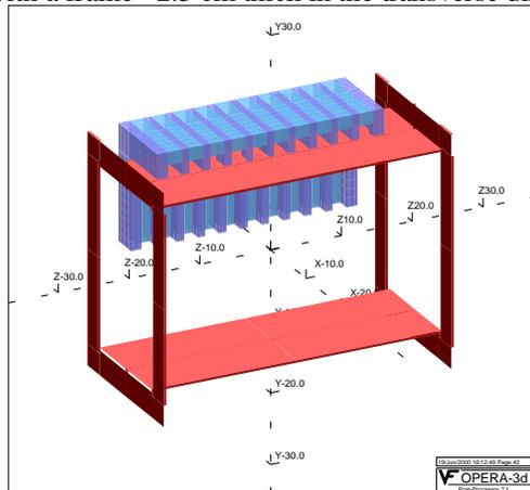
Figure 3: A 3-dimensional view of the kicker. The red material is the copper conductor shown in full. For a good view, of the segmented ferrite (dark-blue 1cm thick in z-dir.) and the material (light blue 2cm thick in z) between the ferrite, only one quarter of the kicker is shown.
