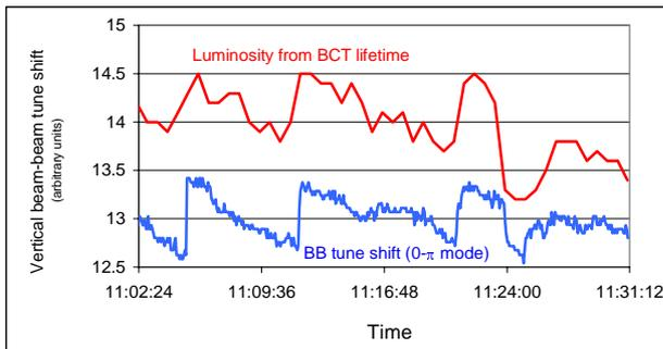
Figure 5: Measured beam-beam tune shift from the  $\sigma$ - $\pi$  mode and luminosity from the BCT versus time.
