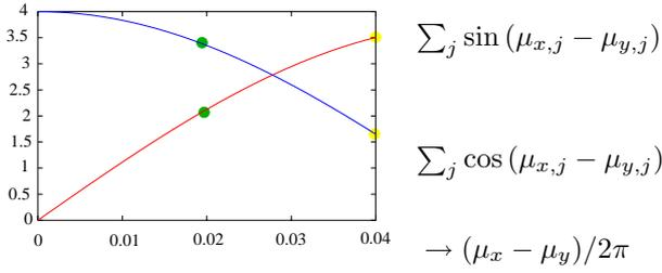
Figure 3:  $\sum_j \cos(\mu_{x,j} - \mu_{y,j})$  and  $\sum_j \sin(\mu_{x,j} - \mu_{y,j})$  as a function of the the tune split per cell. The points on the left indicate the values for the LHC V6.1 with tune split 5 and the points on the right the values for the resonance free lattice (tune split 9)
