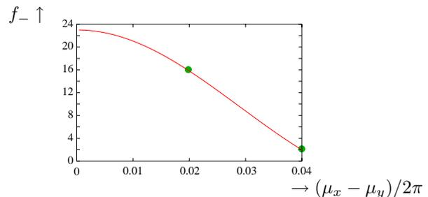
Figure 2:  $f_-$  as a function of the tune split per cell. The points indicate the values for the LHC V6.1 with tune split 5 and 9 (resonance free lattice [1])
