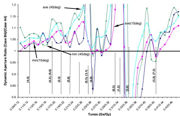
Figure 2: Ratio of short-term dynamic aperture (1,000 turns) (**Case B4**)/(**Case A4**) v.s. tune. Average and minimum ratio over 60 random seeds are given at the phase space angles  $\phi = 15^\circ, 45^\circ$  respectively for each pair of tunes, which are separated by 0.03.
