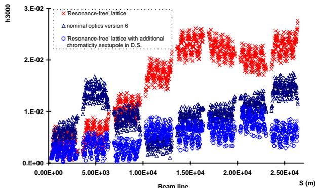
Figure 1: Comparison of the  $3^{rd}$  order resonance driving term  $h_{3000}$  (*random seed 1*) excited along the LHC ring for the resonance-free lattice and the nominal optics version 6 in the absence of  $b_3$  spool pieces. The former is shown with and without extra chromaticity sextupoles in the D.S..
