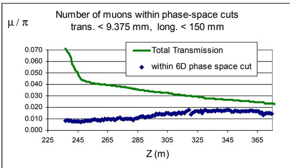
Figure 5: Performance of cooling channel with beam having a too large energy spread coming in.
