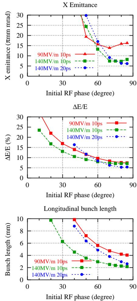
Figure 6: Calculated dependence of emittance, energy spread and bunch length on initial RF phase
