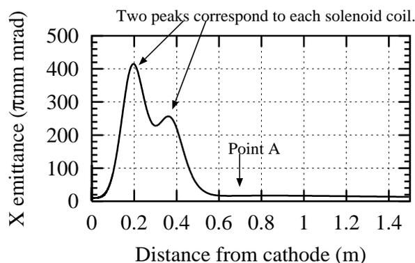
Figure 4: Typical calculated emittance along a beam line
