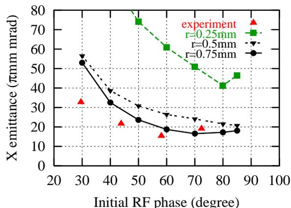
Figure 5: Emittance comparison between experiment and simulation
