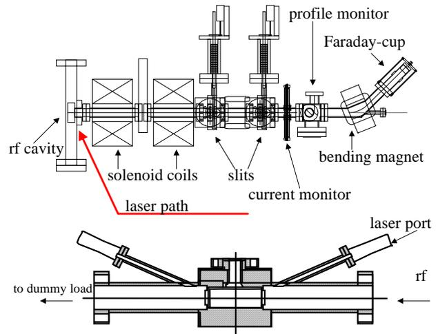
Figure 1: Outline of experiment apparatus
