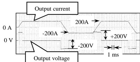
Figure 5 Current Pattern for raster scanning method
