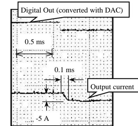
(a) Output current of the power supply
