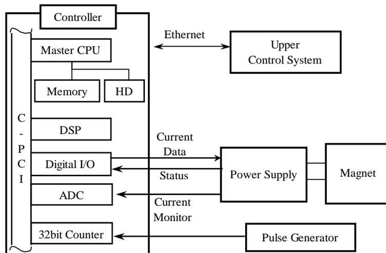
Figure 2 Control system of the power supply for fast pattern excitation
