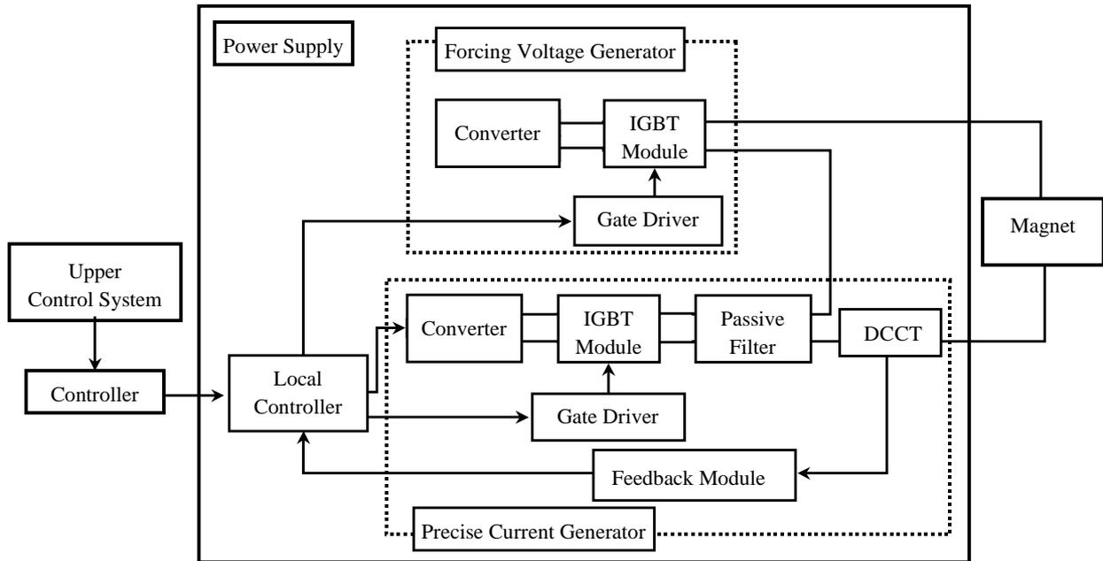
Figure 1 Schematic drawing of the Power supply system for fast pattern excitation
