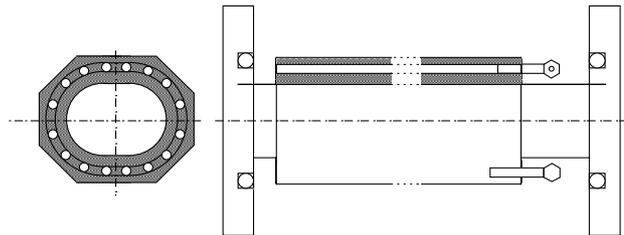
Figure 1: Structure of the ceramic chamber of HER injection kicker
