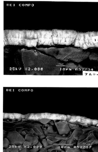
Figure 3: Ti coating thickness (Upper: 3-A Lower: 3-B)
