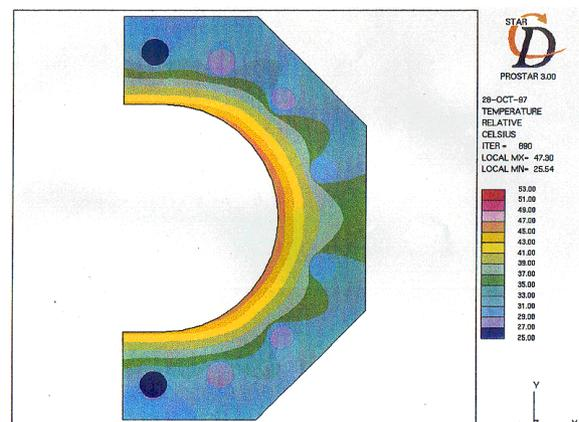
Figure 4B: Temperature of ceramic
