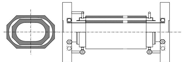
Figure 2: Structure of the ceramic chamber of LER injection kicker
