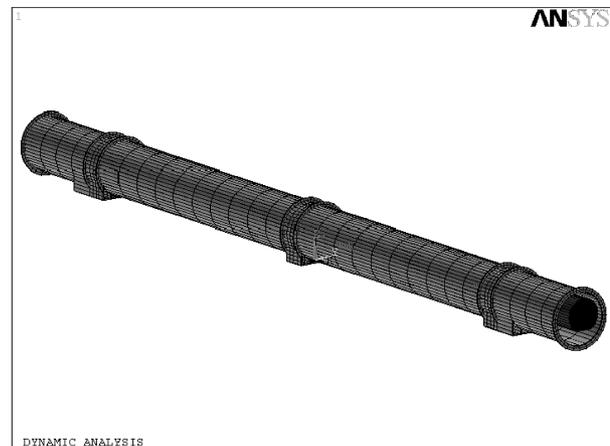
Figure 2: Finite element model of the LHC cryodipole
