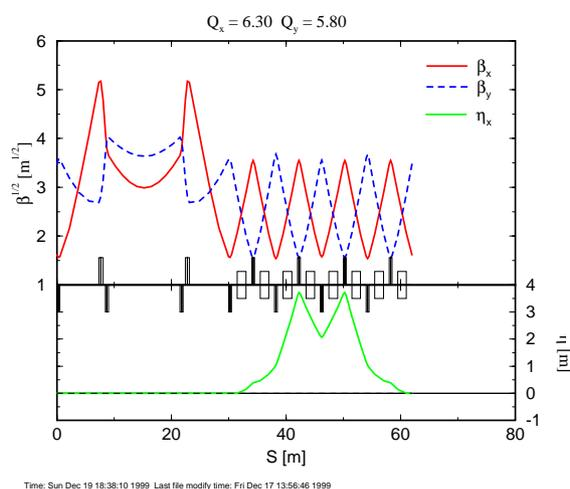
Figure 3: Lattice functions of one lattice super-period consisting of a FODO arc and a doublet straight. The horizontal phase advance across the arc section is  $2\pi$  radian. The dispersion in the straight section is zero.
