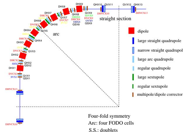
Figure 2: Schematic layout of one lattice super-period.
