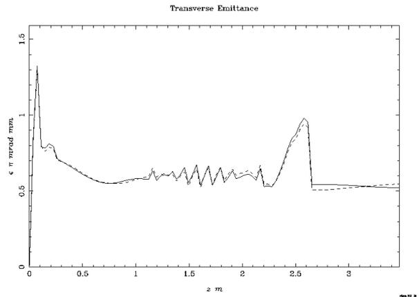
Fig. 2: Horizontal and vertical emittance obtained from ASTRA [5] simulations for the electron source up to position  $z$  just before the end of the solenoid.
