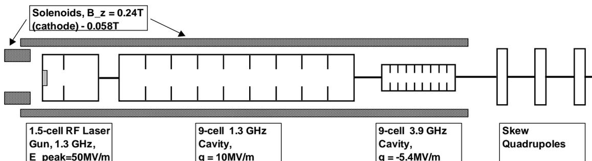
Figure 1: Sketch of the electron beam source layout.
