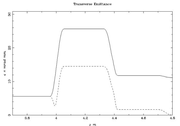
Fig. 4: Evolution of horizontal (full line) and vertical (dashed line) beam emittance through the adapter section.
