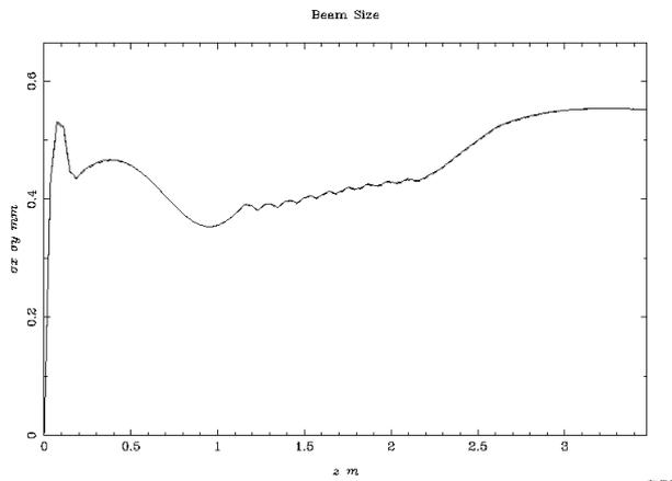
Fig. 3: Transverse beam size in the electron source beam line up to the end of the solenoid.
