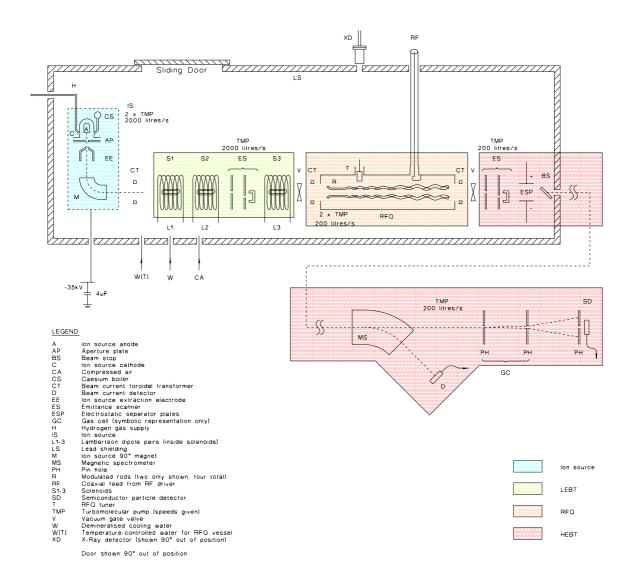
Figure 1: Functional outline drawing of the Rutherford RFQ Test Stand. The drawing is intended to show only the essential components of the RFQ Test Stand, and is not to scale.
