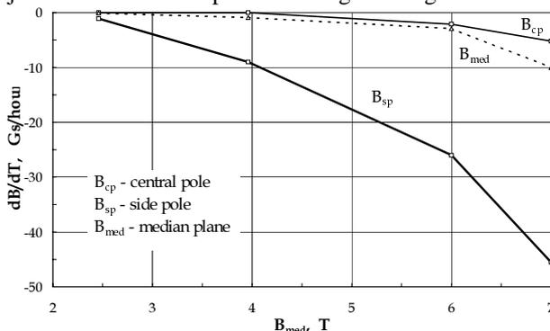
Fig. 5: Dependence of the rate of field degradation on the wiggler field value.
