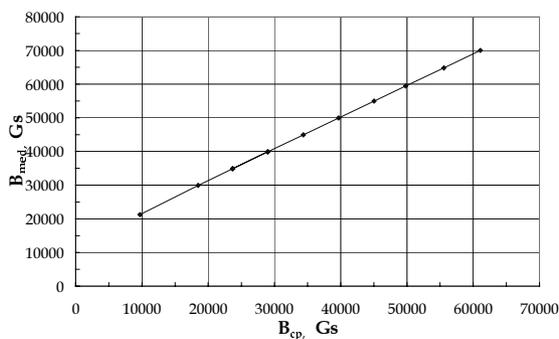
Fig. 3: Dependence of the field value in the median plane  $B_{med}$  upon the field value in the central pole  $B_{cp}$ .
