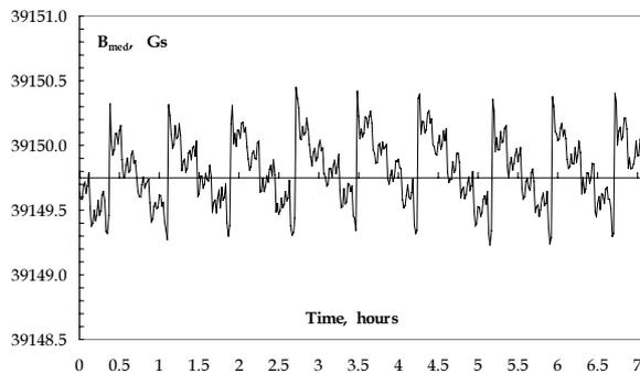
Fig. 7: Field stabilization for wiggler field value  $\sim 4T$ .
