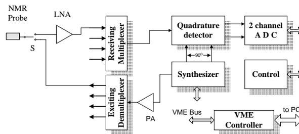
Fig. 4: A simplified scheme of the NMR System. PA - power amplifier, LNA - low noise amplifier, S - receiving/exciting switch.
