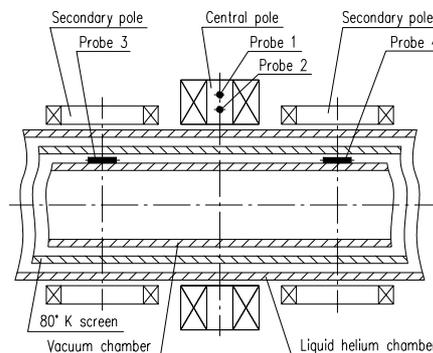
Fig. 1: The draft of the Wiggler and NMR probes locations.
