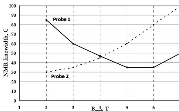
Fig. 2: Dependence of the resonance linewidth upon the Wiggler field value in the median plane.
