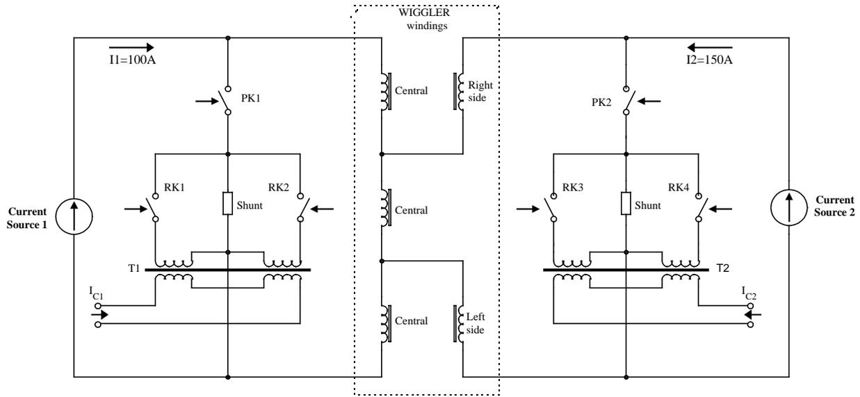
Fig. 6: A simplified scheme of current pumping system for field stabilization.
