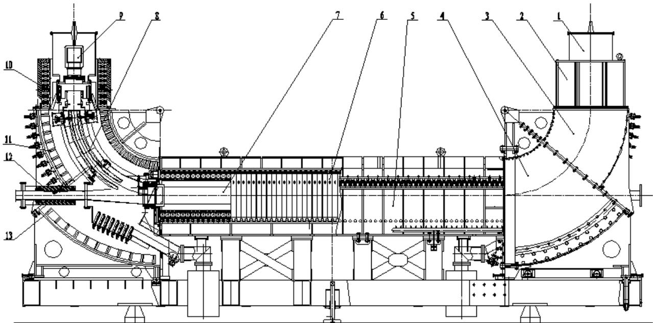
Figure 1: General arrangement of the EX-35 electron cooling device at an electron energy of 35 keV. 1-electron gun, 2-gun solenoids, 3-toroid 40°, 4-toroid 50°, 5-main solenoid, 6-main solenoid coil, 7-vacuum chamber, 8-electrostatic deflector, 9- collector, 10-collector solenoids, 11-toroid 40° coil, 12- correcting magnet, 13-toroid 50° coil.
