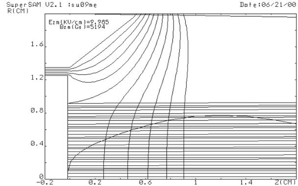
Figure 3: Decreasing of the emitting diameter at  $-2.5$  kV voltage at the control electrode.
