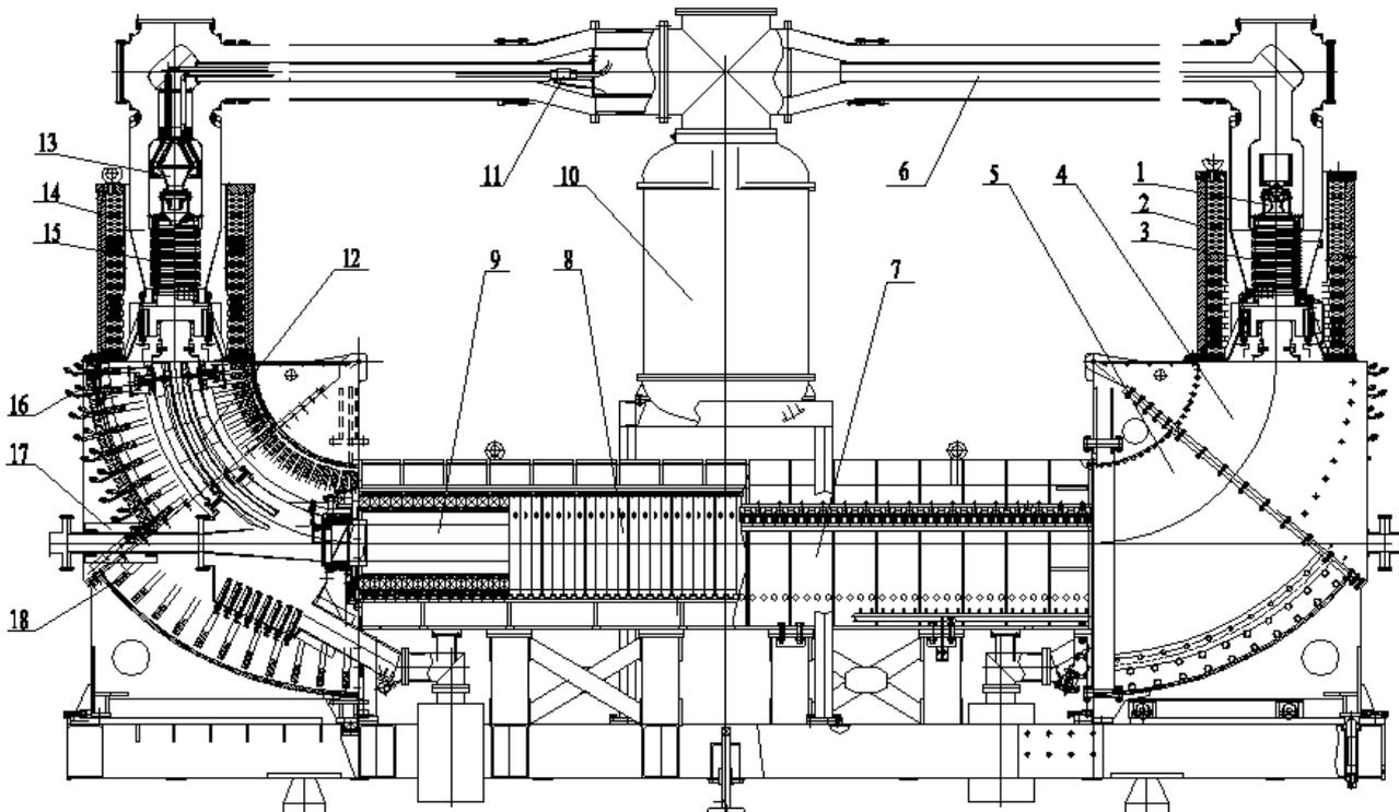
Figure 2: General arrangement of the EX-300 electron cooling device at an electron energy of 300 keV. 1-electron gun, 2-gun solenoids, 3- accelerating tube, 4-toroid 40°, 5- toroid 50°, 6- SF<sub>6</sub> high voltage feeder, 7-main solenoid, 8-main solenoid coil, 9-vacuum chamber, 10-300 kV rectifier, 11-collector cooling system, 12-electrostatic deflector, 13- collector, 14-collector solenoids, 15- decelerating tube, 16- toroid 40° coil, 17- correcting magnet, 18- toroid 50° coil.
