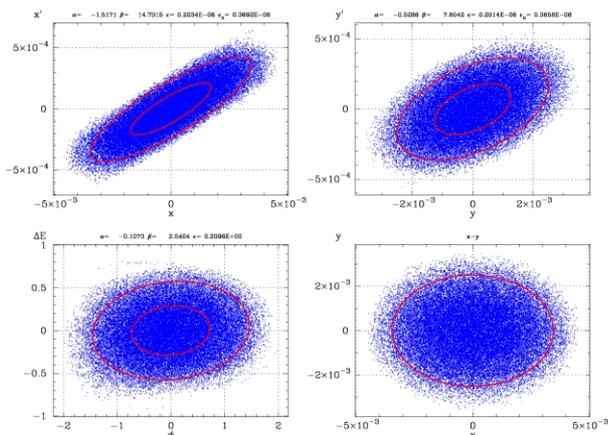
Figure 6: Output beam at 1 GeV (50 k particles simulation). Units are meters and radians for the transverse phase space, degrees and MeV for the longitudinal phase space.
