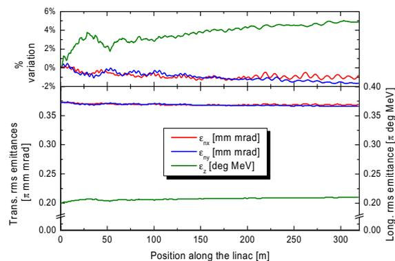
Figure 3: rms normalized emittances in the linac.
