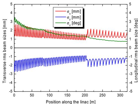
Figure 2: rms beam sizes in the matched SC linac, up to 1 GeV, from the multiparticle simulations.
