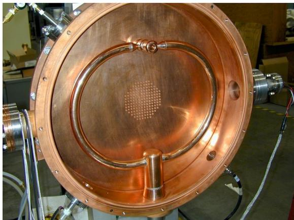
Figure 5. DTL Buncher developed and manufactured at INR, Russia.
