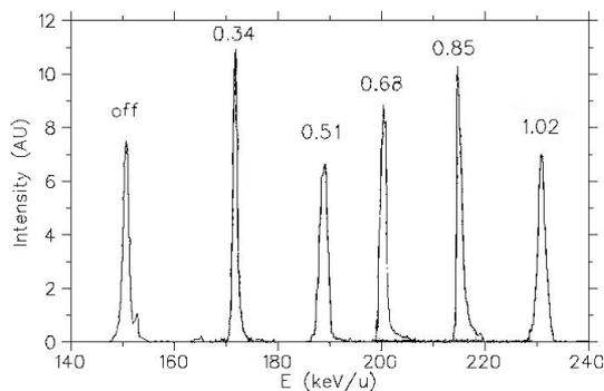
Figure 6. Final beam energy for various DTL tank1 amplitude settings.
