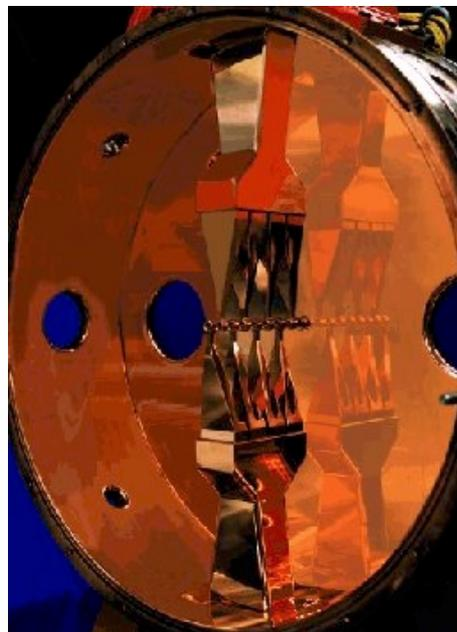
Figure 4. First DTL tank with ridges and stems installed.
