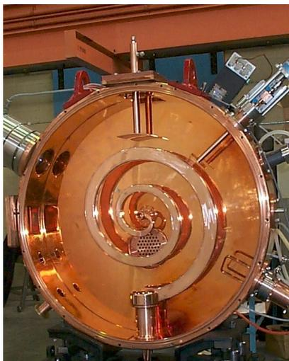
Figure 3. MEBT Spiral Re-buncher.
