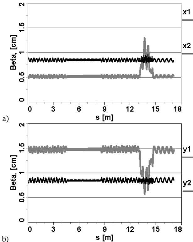
Figure 3.  $\beta_x$  (a) and  $\beta_y$  (b) functions for two invariants of motion.
