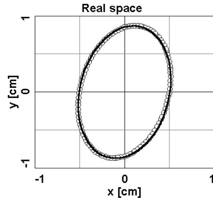
Figure 1. The particle trajectory in the transverse plan of real space at the initial point of storage ring ( $s=0$ ). Circle points are the result of tracking, solid line - phase ellipse calculated using  $\mathbf{A}$  matrices.
