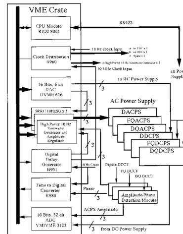
Figure 1: Block diagram of the booster power supplies control interface
