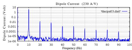
Figure 6: Spectrum of Dipole Current.
