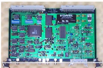
Figure 3: Photograph of the 10 Hz sinusoidal generator and amplitude regulator.
