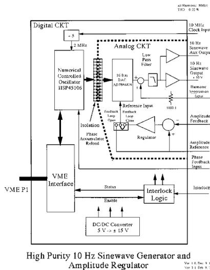
Figure 2: Block diagram of the 10 Hz high purity sine-wave generator and amplitude regulator.
