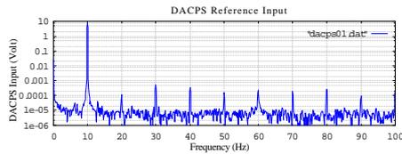
Figure 4: Output spectrum of 10 Hz signal generator.
