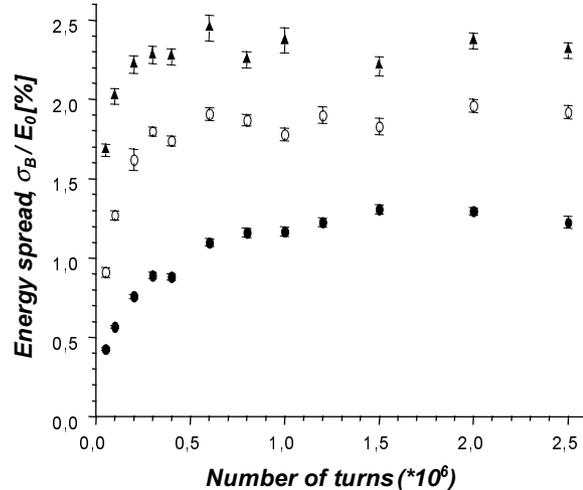
Figure 3. The electron beam energy spread versus turn number. Solid circles -  $E_0=40$  MeV, open circles -  $E_0=100$  MeV, triangles -  $E_0=200$  MeV.
