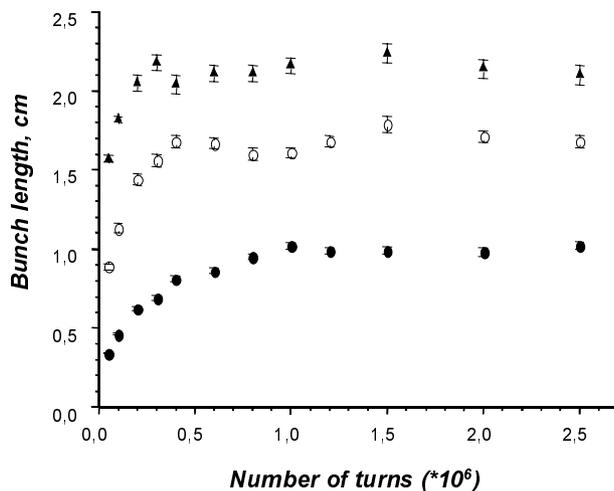
Figure 2. The electron bunch length versus turn number. Solid circles -  $E_0=40$  MeV, open circles -  $E_0=100$  MeV, triangles -  $E_0=200$  MeV.
