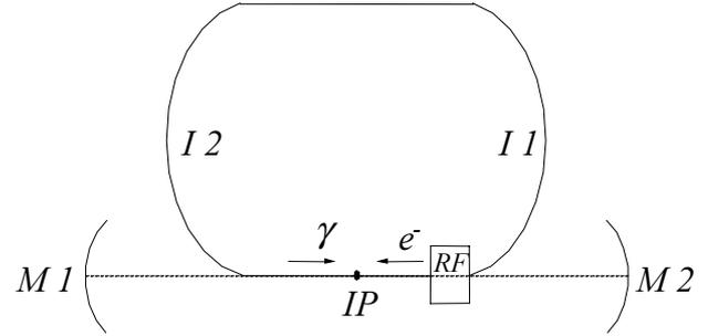
Figure 1. The scheme of the ring used in simulations. Figure captions:  $RF$  – the  $RF$ -cavity;  $IP$  – the interaction point for the electron and laser beams;  $M1$ ,  $M2$  – the mirrors of the optical resonator.
