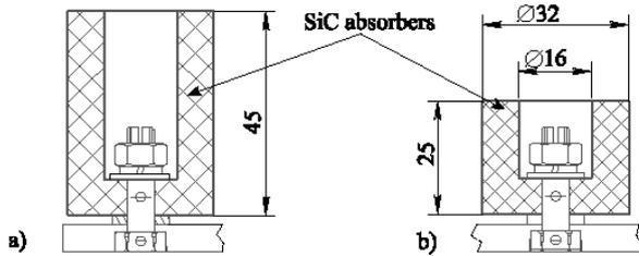
Fig.2. Absorbing element a) of the coaxial HOM load, b) of the waveguard HOM load.
