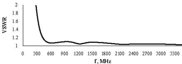
Fig.3. VSWR of coaxial load calculated by SUPERFISH.
