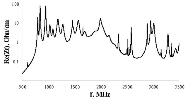
Fig.5. Dipole mode spectrum of the single mode cavity.
