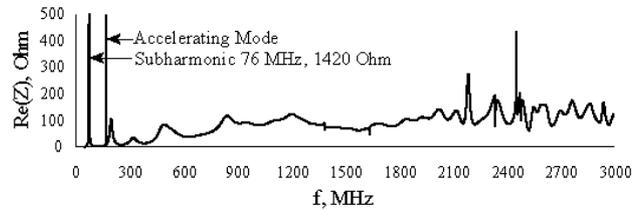
Fig.4. Real part of coupling impedance of HOM of cavity
