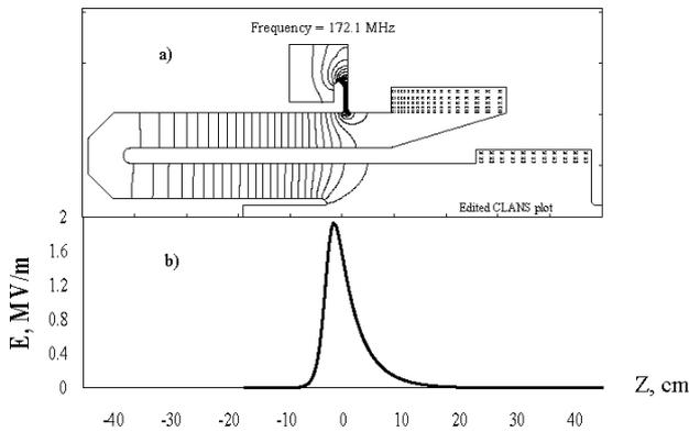
Fig.6. a) Close view of the field pattern of the accelerating mode. After the choke filter TEM mode transforms to  $E_{01}$  mode and do not propagate to the load, as the critical frequency of  $E_{01}$  mode in the coaxial waveguide is more higher then accelerating frequency.
