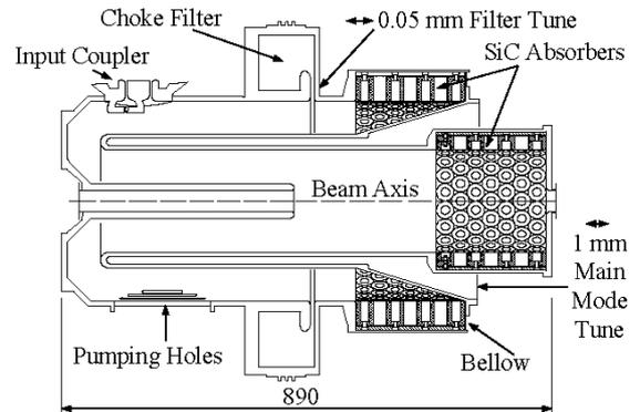
Fig.1. Schematic drawing of the single-mode cavity.
