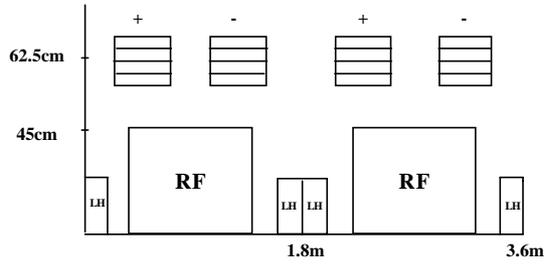
Figure 1: Configuration of the DFOFO cooling channel which has 1.8m cell long. RF cavities of pillbox type with 5-cell structure are used. Al window is used to sustain the liquid hydrogen. Sheets with 50 cm long and 15cm height are used to generate realistic magnetic fields.
