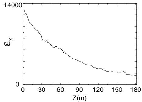
Figure 4: X-dimensional emittance ( $mm-mrad$ ) vs.  $Z$ (m) in the DFOFO cooling channels
