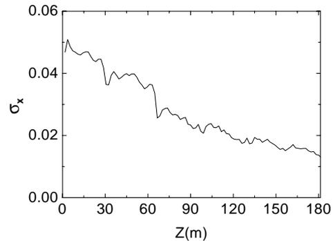
Figure 5: RMS beam size  $\sigma_x$  (m) vs.  $Z$ (m) in the DFOFO cooling channels
