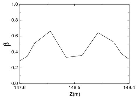
Figure 3: Beta function ( $\beta_x$ ) vs.  $Z$ (m) in one cell of second stage DFOFO cooling channel..
