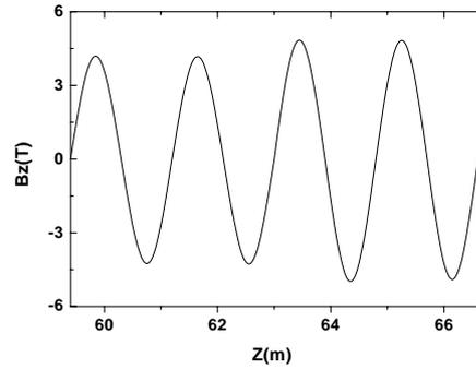
Figure 2: Magnetic field ( $B_z$ ) vs.  $Z$ (m) in interface of first and second DFOFO cooling channels. The magnetic field has minimum values in the midpoint of rf cavities.
