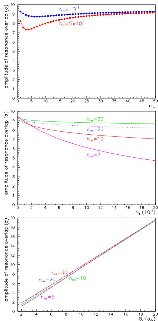
Figure 5: Minimum amplitude at which the overlap condition Eq. (1) is fulfilled as a function of [top] resonance order  $n_{\text{res}}$  (for  $\theta_c \approx 9.5\sigma'_{\text{ip}}$ ,  $N_b = 1.05 \times 10^{11}$ ), [center] bunch population (for the same crossing angle and five different resonance orders) and [bottom] crossing angle  $\theta_c$  (for the nominal bunch population  $N_b = 1.05 \times 10^{11}$  and four different resonance orders).
