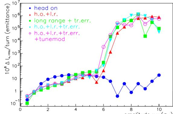
Figure 1: The change of action variance per turn as a function of starting amplitude in the LHC with  $9.5\sigma'_x$  separation [1]. Whenever l.r. collisions are present, the diffusion rate increases sharply at about  $6\sigma$ .
