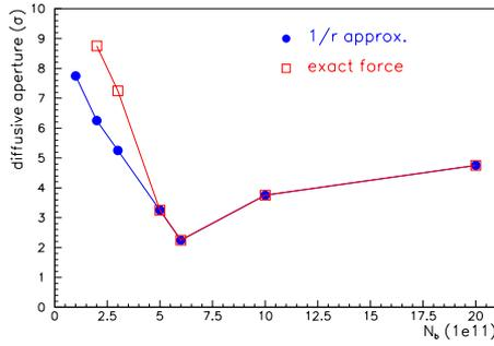
Figure 2: Simulated diffusive aperture as a function of bunch population, for 30 parasitic collision points and  $\theta_c \approx 9.5\sigma_{x'}$ . The figure compares the results for the exact force and those obtained using the  $1/r'$  approximation.
