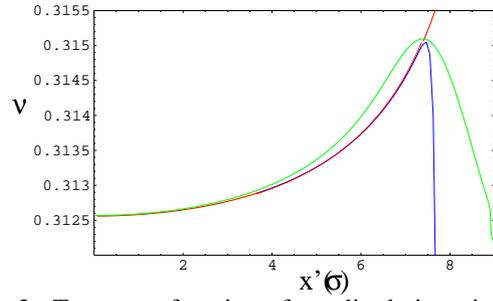
Figure 3: Tune as a function of amplitude in units of  $\sigma'$  due to l.r. beam-beam interaction for a separation of  $9.5\sigma_{x'}$ . Tracking result (green), the  $1/r'$  term only (red), and the  $1/r'$  part plus a single term ( $k = 14, l = 3$ ) in the Bessel expansion (blue).
