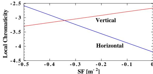
Figure 3: Local chromaticity corrections with focusing sextupole fields
