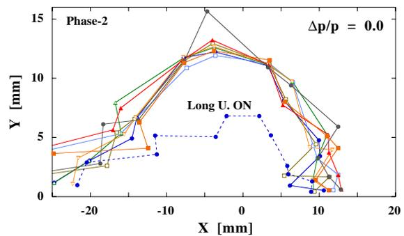
Figure 7: Dynamic apertures of the phase-2 lattice with realistic errors. COD is corrected. Also shown by the dashed curve is the aperture with a long undulator (example case).
