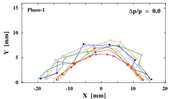
Figure 6: Dynamic apertures of the phase-1 lattice with realistic errors (typical cases). COD is corrected.
