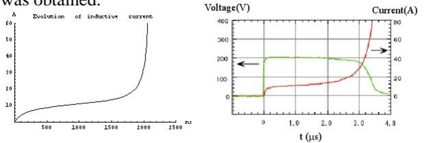
Figure 2: Magnetic current estimated and measured
