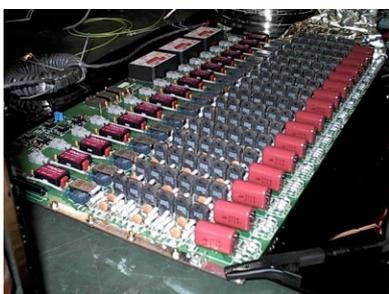
Figure 6: The FET switching array
