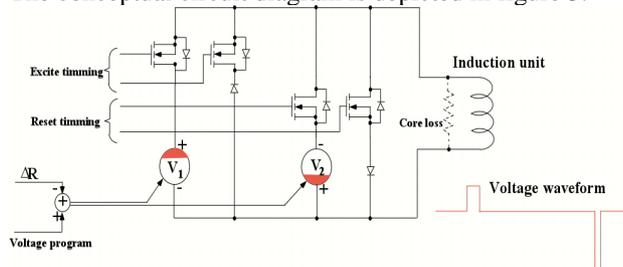
Figure 5: A conceptual design of the switching unit
