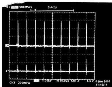
Figure 7: 100kHz continuous operation result. Upper trace is the voltage waveform Lower trace is the current in to the core.
