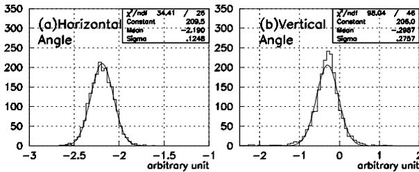
Figure 4-(a) and (b): The canonical crossing angles between the two beams during a fill.
