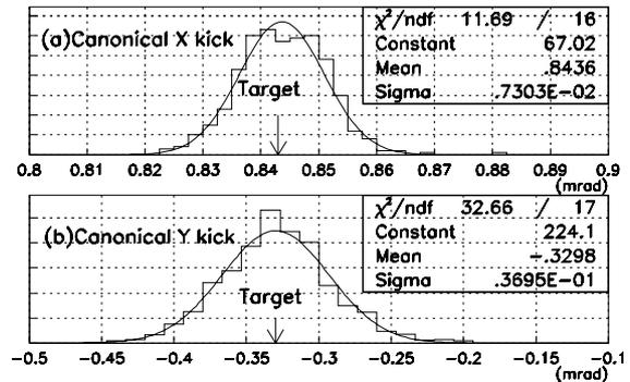
Figure 3: (a) The canonical horizontal kick distribution when the target value was 0.843 mrad; and (b) the canonical vertical kick distribution when the target value was -0.33 mrad during Fill 1677.
