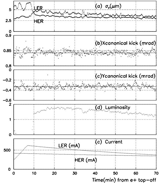
Figure 2: Fill 1677 trend graph, (a) HER and LER vertical beam sizes, (b) horizontal canonical kick and the target values, (c) vertical canonical kick and the target values, (d) Luminosity ( $\times 10E32/\text{cm}^2/\text{s}$ ) and (e) HER/LER beam currents are plotted against time (minutes) measured from the beginning of positron top-off.
