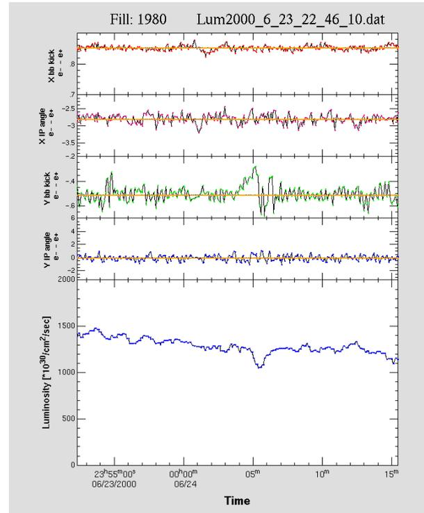
Figure 5: Top four plots correspond to the canonical horizontal kick, horizontal crossing angle, vertical kick and vertical crossing angle, respectively for Fill 1980. Luminosity( $\times 10^32/\text{cm}^2/\text{s}$ ) is plotted at the bottom.
