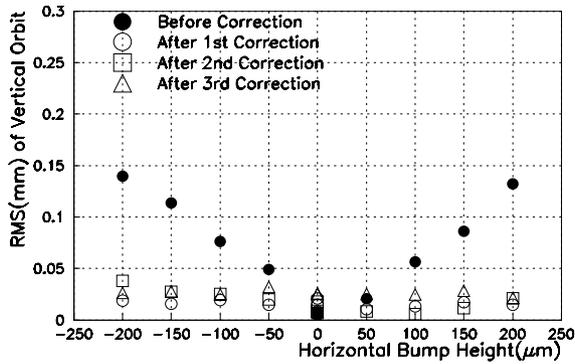
Figure 1: The calibration of the horizontal-vertical coupling from the iBump. After correction, the coupling effect is negligible.
