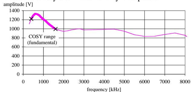
Fig. 7: Cavity voltage for -3dBm amplifier input.
