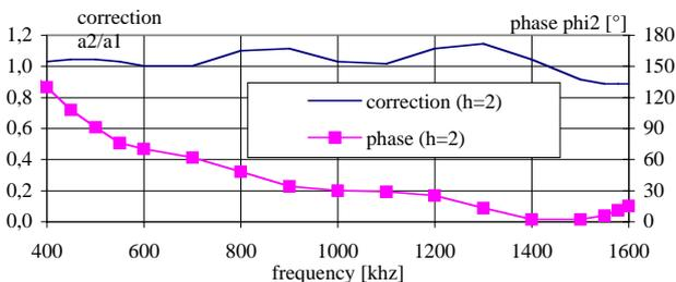
Fig. 10: Measured phase and amplitude relation between harmonics ( $h=1$ ) and ( $h=2$ )
