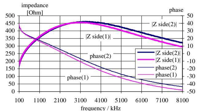
Fig. 3: Impedance of both sides of VitroPerm cavity filled with air
