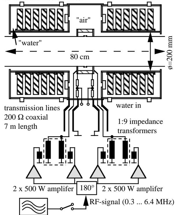
Fig. 6: Layout of cavity, transmission lines, transformers and amplifiers
