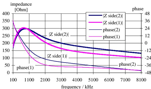
Fig. 5: Impedance of both sides of low-conductive water-filled VitroPerm cavity; second assembly
