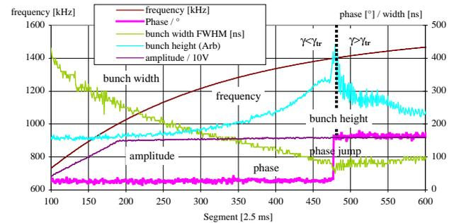
Fig. 11:  $\gamma$ -transition crossing at COSY with ferrite cavity and adjusted phase-jump
