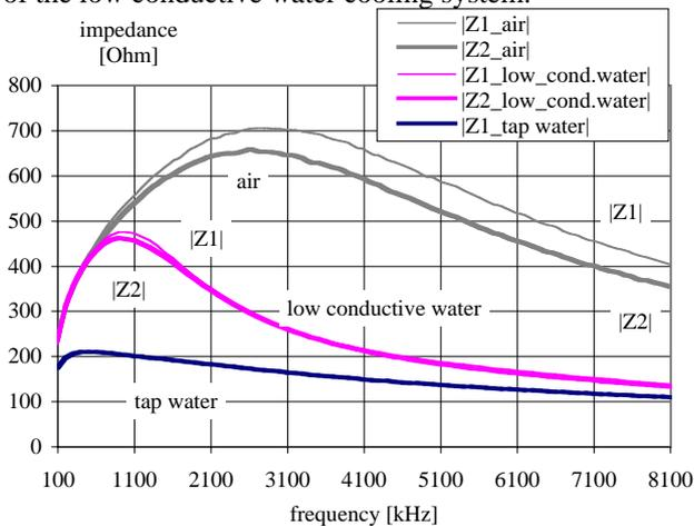
Fig. 1: Impedance as function of cooling medium, measured on both cavity sides 1 and 2 separately
