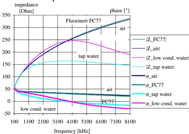
Fig. 4: Impedance of 3 VitroPerm sample cores as function of cooling medium
