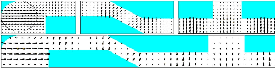
Figure 3: Electric field of the  $f = 1.50325$  GHz-eigenmode computed using CSC (upper) and MAFIA-E (lower). (Jumps in vector size are artificially introduced by different display scalings).
