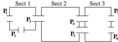
Figure 1: A rf-system of three sections with external ( $P_1, P_2, P_6, P_7$ ) and internal ports ( $P_3, P_4, P_5$ )
