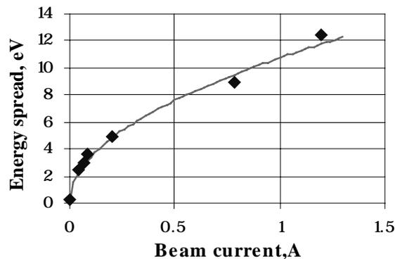
Figure 5: Energy spread as a function of the beam current. Magnetic field is 2 kG, solid line corresponds to the fit  $\delta W[eV] = 10.8 \cdot \sqrt{I[A]}$ .
