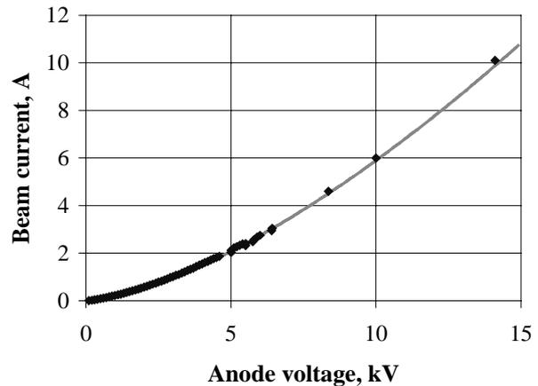
Figure 3. Beam current as a function of the anode voltage. Magnetic field is 2 kG,  $U_{ce} = 0$ . Diamonds represent experimental points, and the solid curve shows the fit with  $P = 5.9 \mu A / V^{3/2}$ .
