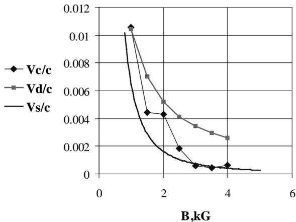
Figure2: Results of simulation of the drift and cyclotron components at  $U_a = 10$  kV,  $I = 5$  A without taking into account electron thermal velocities. The curves represent maximum values throughout the beam in the drift tube.
