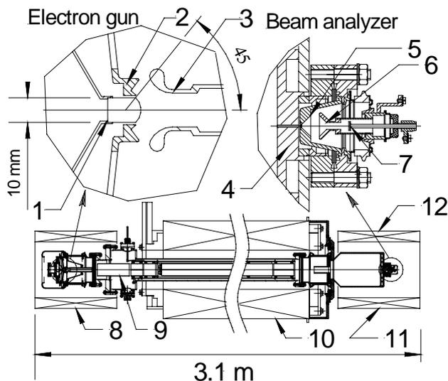
Figure 1: Mechanical schematic of the test bench. Electron gun and the beam analyzer are shown in detail. 1- cathode, 2- control electrode, 3- anode, 4- water-cooled collector bottom with a 1mm hole in the center, 5- diaphragm with 0.6 mm hole, 6- retarding electrode, 7- analyzer collector, 8- gun solenoid, 9- drift tube, 10- main solenoid, 11- collector solenoid.
