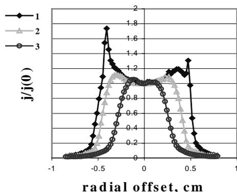
Figure 4: Current density distributions for three control electrode voltages: 1-  $U_{ce} = 0$ ,  $I = 1$  A; 2-  $U_{ce} = -0.3$  kV,  $I = 0.6$  A, 3-  $U_{ce} = -1.2$  kV,  $I = 0.16$  A.  $U_a = 3$  kV, magnetic field in all solenoids 2 kG.
