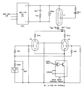
Figure 1: Basic Diagram of the Solid-State Deck
