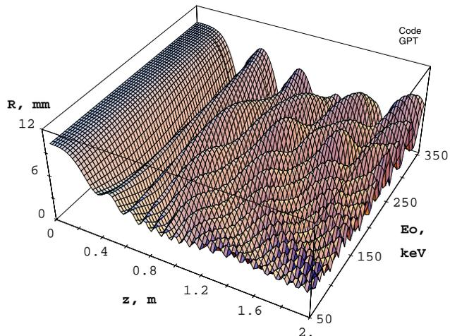
Figure 4: Trajectories of the particles with different energies in a mixed guiding field. The longitudinal axis corresponds to the longitudinal position, the transverse axis - the particle energy, vertical - to the radius of the trajectory.
