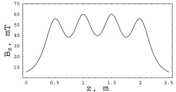
Figure 3: Profile of the longitudinal magnetic field formed by an array of real magnetic lenses.
