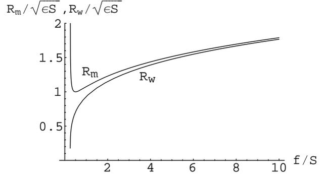
Figure 2: Dependence of the maximum beam radius  $R_m$  (upper curve) and the beam radius in the waist  $R_w$  (lower curve) on the ratio  $f/S$ .
