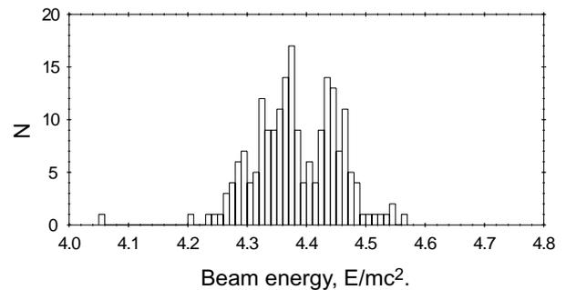
Figure 1: Energy spectrum of the electron beam at the FEM undulator exit.
