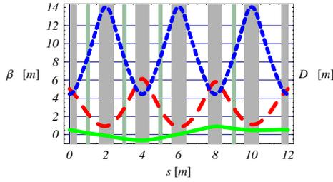
Figure 1: Horizontal (dashed line) and vertical (dotted line)  $\beta$ -functions and orbit dispersion (solid line) in an isochronous period.
