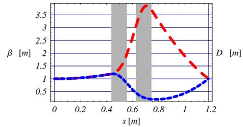
Figure 4: Horizontal (dashed line) and vertical (dotted line)  $\beta$ -functions for a symmetrical doublet with finite length quadrupoles of 12 cm.  $\beta_h = \beta_v = 1.15955$  m,  $\alpha_h = -\alpha_v = 2.34717$ .
