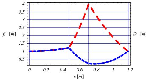
Figure 2: Horizontal (dashed line) and vertical (dotted line)  $\beta$ -functions for a symmetrical doublet made of thin lenses.
