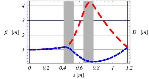
Figure 3: Horizontal (dashed line) and vertical (dotted line)  $\beta$ -functions for a symmetrical doublet with finite length quadrupoles of 12 cm.  $\beta_h = 1.0005$  m,  $\beta_v = 1.0004$  m,  $\alpha_h = 2.0009, \alpha_v = -2.0009$ .
