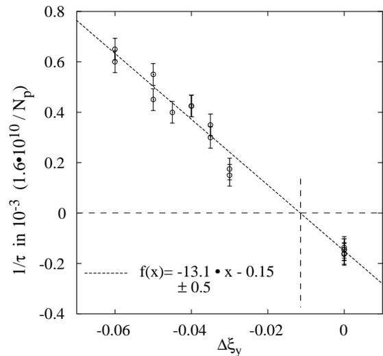
Figure 2: 10/11/1999. Growth rate of the vertical head-tail mode instability (in units of  $10^{-3}$  turns $^{-1}$ ), as a function of the decrement of chromaticity. Error bars are  $e = 0.043$  (in units of  $10^{-3}$ ).
