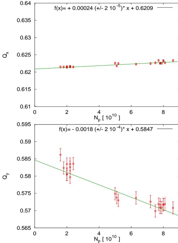
Figure 1: 13/08/1999 ( $V_{rf}=0.8$  MV). Horizontal (top) and vertical (bottom) tune as a function of the bunch population and fit with errors. Tune error bars  $e_y = 1.8 \times 10^{-3}$  and  $e_x = 3 \times 10^{-4}$ .
