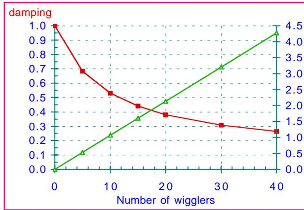
Figure 4: Effects of damping wigglers on emittance and on energy loss per turn increase
