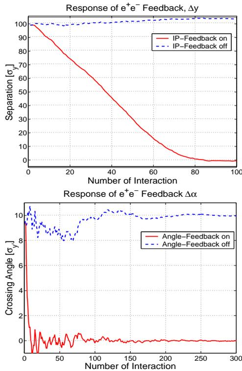
Figure 4: Response of the beam separation and angle feedback to an initial crossing angle of  $10\sigma_{y'}$  and beam separation of  $100\sigma_y$ . Noise sources listed in section 4 are taken into account. The luminosity is kept beyond 90%.
