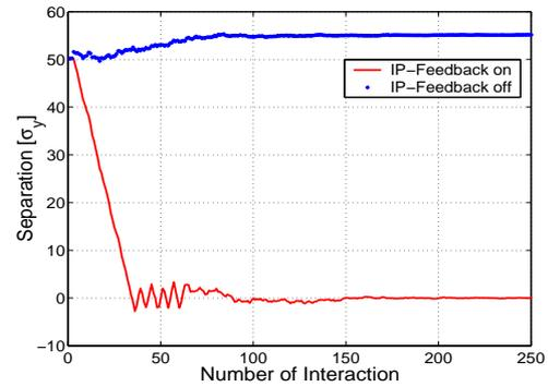
Figure 5: Response of the  $e^-e^-$  separation feedback to an additional beam separation of  $50\sigma_y$ .
