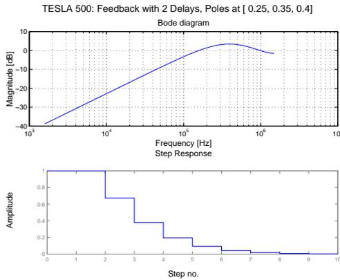
Figure 1: Frequency and step response of intra-train feedback system in TESLA.
