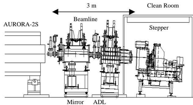
Figure 5: Schematic of compact beamline for X-ray Lithography.
