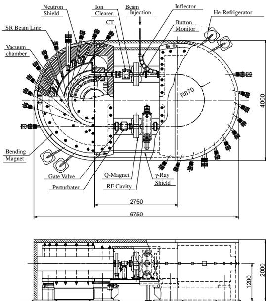
Figure 2: Schematic of A2S.
