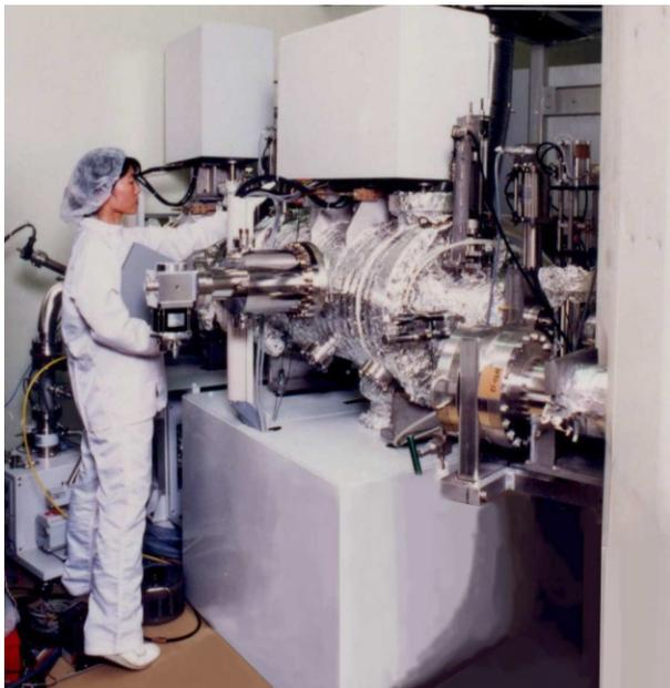
Figure 6: Photo of compact beamline for X-ray litho.
