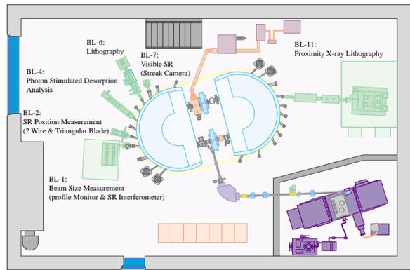
Figure 4: Layout of A2S prototype (Injector, BT, storage ring, etc.) and experimental setup.
