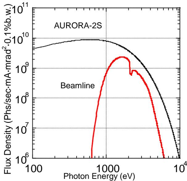
Figure 3: X-ray spectra of A2S and beamline.
