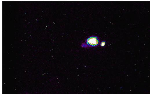
Figure 7: 0.5 mm HeNe laser (large one) and OTR image of electron beam for 0.3 nC charge.
