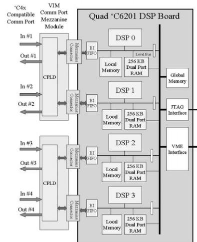
Figure 3: DSP hardware I/O port.
